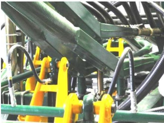
By increasing the primary hose length and keeping the secondary hose to an acceptable length, will result in a more suitable air pressure to fan rpm relationship. This effectively gives the air seeder a greater potential to reach its maximum capacity.
