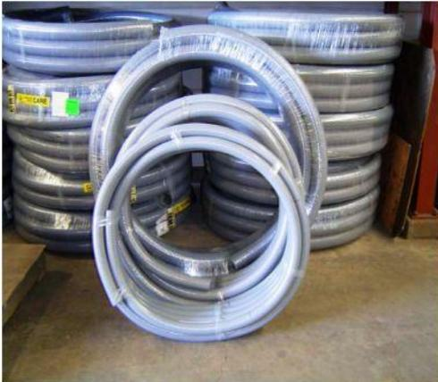
**Primary Lines:** These are the hoses that carry product from the Airseeder metering units to the Primary Dividers. This hose is always 76mm internal diameter and has a smooth hard interior.
