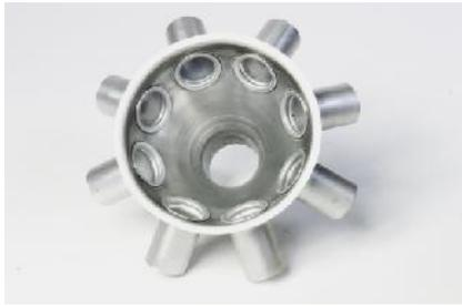
Secondary Heads can have either a 44.5mm or 50mm base to suit the uptube. This size is determined by the primary divider outlet required. Secondary heads can be supplied with 4 to 10 outlets per head. Numbers over 10 or fewer than 4 can not be supplied. The outlets in the secondary heads are always 32.5mm outside diameter to suit above mentioned tertiary hose. All Secondary heads are made from Stainless Steel for durability.
