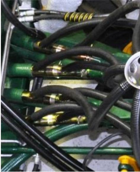
Small seeds induction tubes allow for small seeds to be blended with the main system product at the Primary Divider outlets. The blended products then travel via the secondary lines and heads to the sowing boot to be placed in the ground together.
