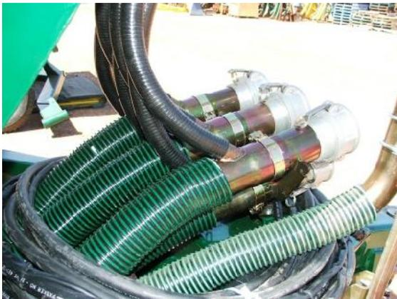
Injection Seeding kit allows product from the small seeds box to be directly injected into the main seeding lines before the seeder camlocks.
