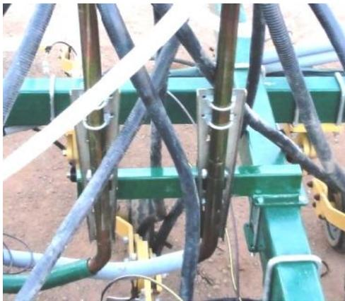
Secondary Heads may need to be staggered, or mounted forward or behind bar on double fold bars to allow for folding.
