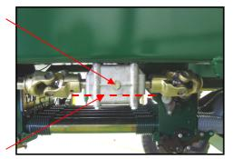
The oil level in each 'T' Box should be checked at the start of the sowing season.
