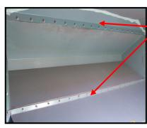
The bin dividers must be fully sealed with silicon as air leaks internally between the bins can be detrimental to the accuracy of the sowing operation. Refer Page 5.1
