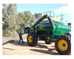
**Step 2**Lift the auger and slide into the rear mount
