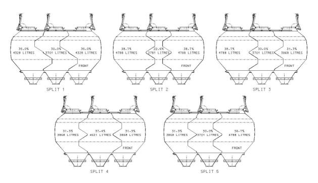
TOTAL USEABLE VOLUME GIVEN A 25 DEGREE ANGLE OF REPOSE IS 12357 LITRES
