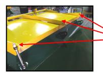
Further adjustment is available by tightening the lock nuts on the hinges.
