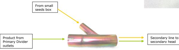
Small seeds induction tubes are a convenient way to place small seed from the small seeds box (option) into the main air streams with the primary product being applied. The blended products then travel via the secondary lines and heads to the sowing boot to be placed in the ground together.
