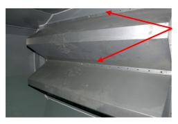
Remove the retaining bolts from around the bin divider/s to be removed and remove the divider/s.
