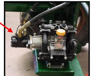
The pump should not be rotated faster than 540rpm. Irreparable damage can result to the pump if operated over 540rpm. To protect against this a flow limiting valve is fitted. This limiting valve simply limits the oil supply to the hydraulic motor so as to deem it impossible to over-rev the pump. This valve is factory set and should not be tampered with. If greater than 540rpm is able to be achieved your Simplicity dealer should be contacted immediately to rectify.
