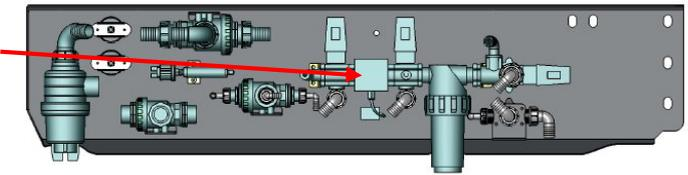
Simplicity Australia fits a 5 to 100 litre per minute flow meter. It is pre-set to produce 600 pulses per litre. Calibration of the flow meter 'fine tunes' this number of pulses per litre to improve accuracy. It is not unusual to have to adjust the flow meter up to 10% either way during this process to account for product variances.
