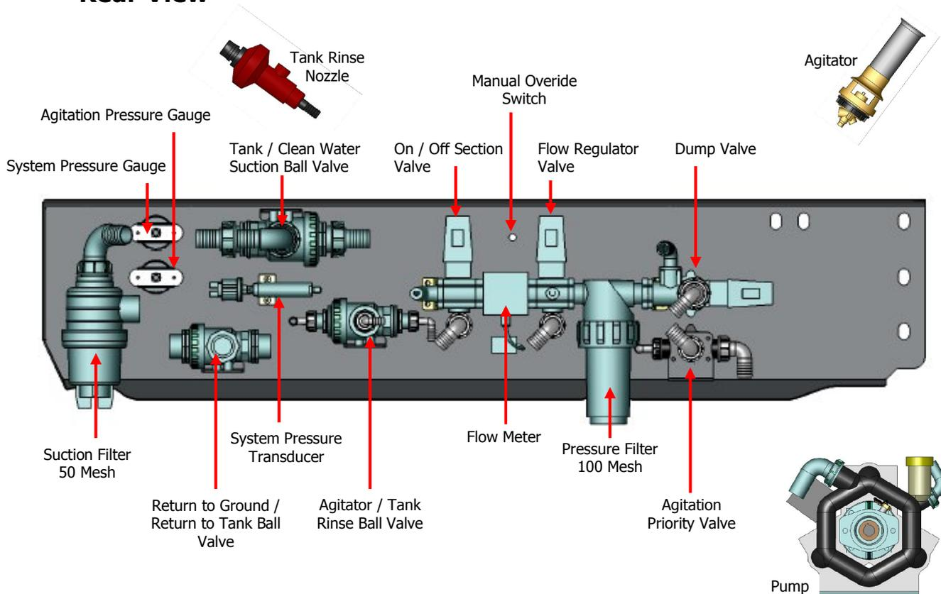
**Pump-** Polypropylene 2136VS Millennium Series Bertolini positive displacement pump. Maximum flow of 120 L/min at 540 rpm. Coupled to a 41cc hydraulic motor the pump has a maximum oil flow requirement of 22 L/min
