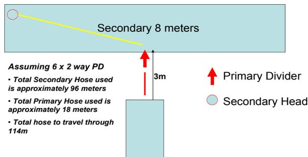
The diagram on the left shows a primary divider fitted at the centre rear of the cultivator. In this example, with a wide implement, the secondary hoses will be far in excess of the recommended five metres. In this case the primary dividers should be moved out further onto the implement, positioned as not to clash with folding, and as shown in the example below.
