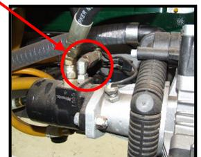
Should the flow limiting valve close due to excessive flow, the hydraulic system must be neutralised then floated to relieve pressure from the circuit. Flow should then be reduced accordingly and then the hydraulic circuit can be re-engaged.
