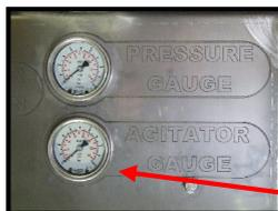
To set simply run pump at required speed and flow, (to begin use 300 rpm), then adjust the Agitator Priority Valve clockwise to increase agitation pressure and flow. Pressure can be easily noted with referral to the Agitation Pressure Gauge.
