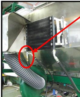
The oil cooler is protected by a relief valve which is pressure set in the factory to divert oil in the case of a pressure build up. A pressure build up is commonly caused by a restriction in the hydraulic return line usually being a quick release coupling being uncoupled.
