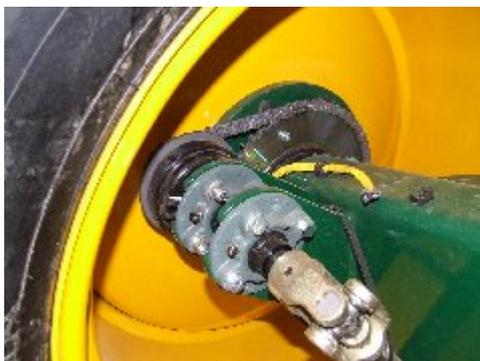
The metering drive system is connected to the drive wheel by an electrically operated mechanical clutch. The clutch requires some maintenance to ensure efficient operation.
